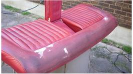
old dye removed and crack filler
