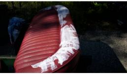
old dye removed and crack filler
