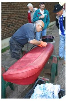
Once the seat has been cleaned and the dye removed then a number of liberal coatings of leatherique rejuvenating oil is applied to soften the leather. 5 Coats a few days apart is optimum. Leatherique recommends that when using their product the use of Pristine Clean preceed the use of the rejuvenating oil to remove embedded dirt and previous layers of dye. These leatherique products are water based.
